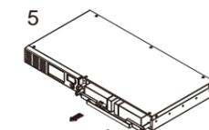
5. Replace the new battery pack. Assemble the screws, cover, and front panel in the reverse sequence of above steps. Recharge the unit for 8 hours to ensure the UPS performs expected runtime.
