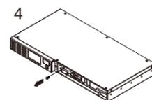
4. Remove the retaining screw of the cable connectors.
