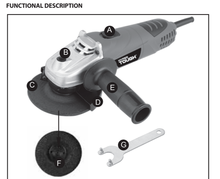
Figure 1 names the major components of the multi-functional tool: A. On/off switch B. Spindle lock button C. Grinding wheel D. Wheel guard E. Side handle F. Outer flange G. Wrench
