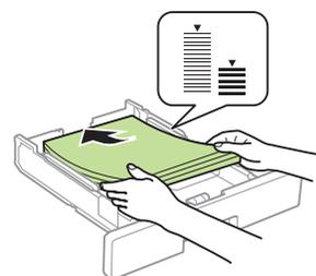
**Note:** Make sure the paper is under the arrow mark for your paper type and loaded against the front edge of the cassette.
