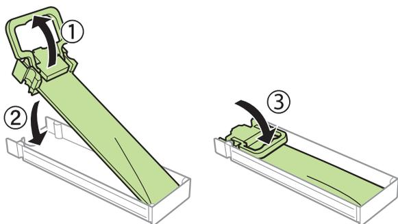
**Note:** Make sure the ink pack is fully inserted and level with the top of the ink pack tray.
