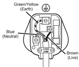
Ensure that the outer sheath of the cable is firmly held by the clamp
