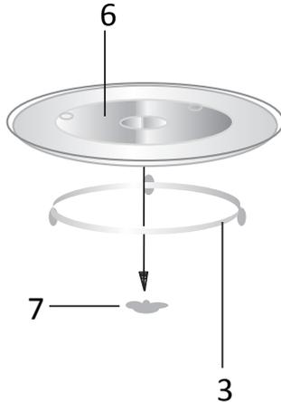
➤ Before first use, check that any securing tape has been removed from the glass tray and turntable ring assembly. These parts must never be restricted from rotating.
