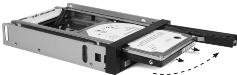
3. Once the drive is fully removed from the drive bay, swing the door closed until it locks in place to prevent damage to the door/hinge. Similarly, the closed door will help prevent dust particles from entering the computer.
