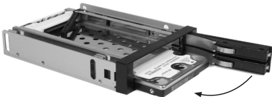
Repeat this procedure to install a second 2.5" SATA drive, into the remaining bay:
