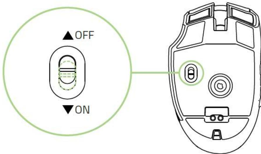
3. To charge the Razer Naga Epic Chroma in wireless mode, ensure that the switch is set to OFF position and then place the mouse on the charging dock.
