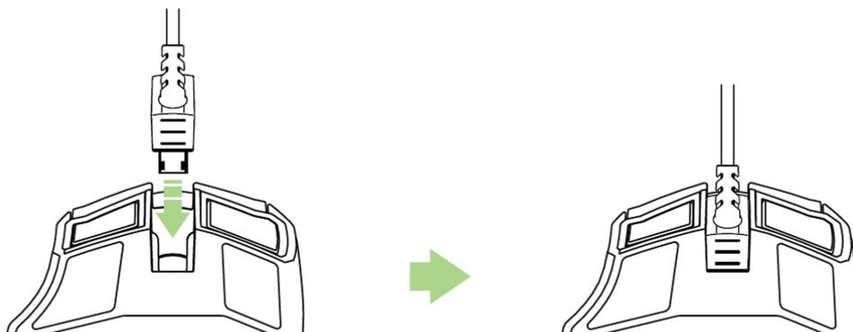
The Razer Naga Epic Chroma is now ready for use as a high performance wired mouse. In addition, its battery will automatically start charging in wired mode.
