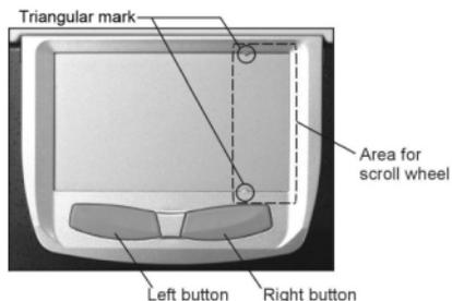
With the keyboard removed, to remove the Touch Pad, pull the small tab underneath it upward to release the latch (1). Slide the touchpad unit forwards (2) until the Touch Pad can be lifted up clear from the notches, as shown in the figure below (3). The Touchpad is connected by a mini-USB cable. To install the Touchpad, connect the mini-USB cable and then slide the Touch Pad all the way in till you hear a click sound as it is locked in position.
