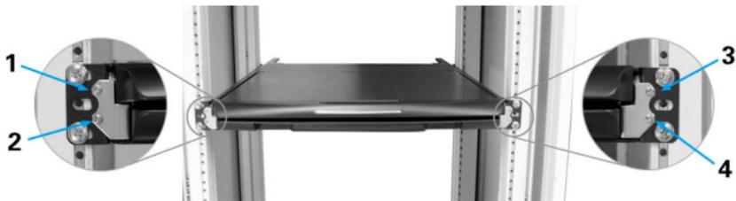
8. Slide the console out slightly until the stoppers along the sides are accessible. Remove the stopper by unfastening the small screws holding it in place.
