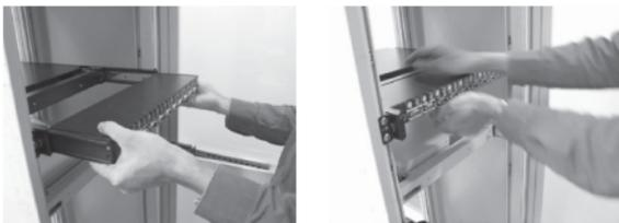
6. Slide the console drawer out and fasten the KVM module together using the screw provided:
