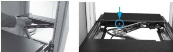
7. Remove the safety stoppers on both sides of the rack console by unfastening the small screws. Please note that once the Safety Stopper is removed, the drawer is free to slide out when the console is tilted. Be cautious, as this could cause injury. Ensure the console is properly installed before removing the safety stoppers.
