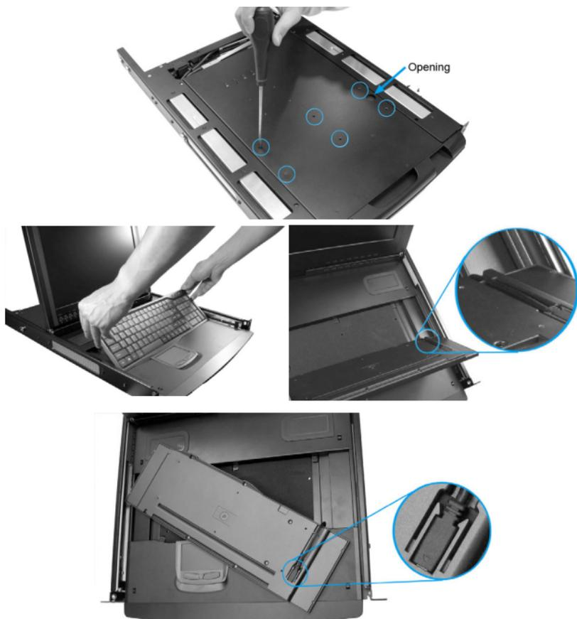
**Please note:** The triangular mark on the mini USB connector must face outwards (be visible).
