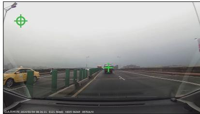
If the calculated intersection is inaccurate, the driver may also perform a manual calibration by pressing the "Image Calibration" button. Upon confirmation of image calibration, the unit's "FCWS" built-in image recognition system can be activated.
