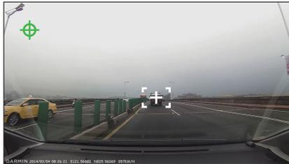
2. If the system detects that the driver is not maintaining an adequate safe distance with the car in front given the current speed, a red cross and frame will be displayed along with a warning sound to alert the driver.
