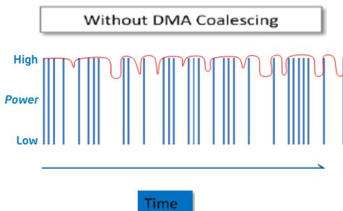
As shown by the red line, components have less time between DMA calls to reach and stay in lower power
