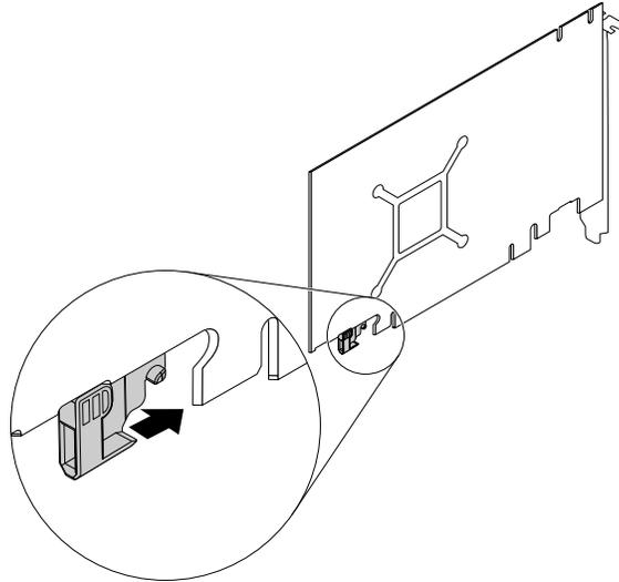
4. Remove the expansion slot cover for the selected expansion slot. Save the screw if there is one to use with the mounting bracket of the graphics card.
