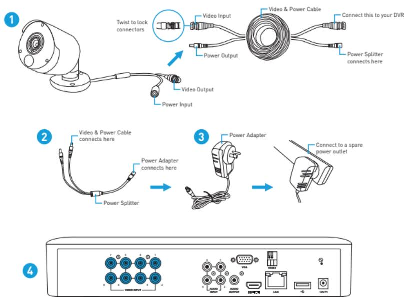
For single camera packs, connect the supplied power adapter directly to the power input on the video & power cable.
