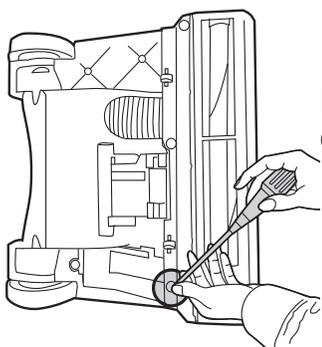
Remove the screws completely.
