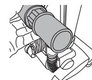
If cleaning tools were in use, check cleaning tool. Next check hose handgrip.
