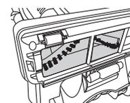
Check that the brushes are free of debris and can rotate.
