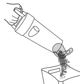
The dust container door will open and you can empty with no contact with dust.
