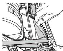
Rotate the brush to ensure free movement of the belt.
