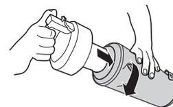
Turn the dust container lid anti-clockwise to unlock and lift to take out.
