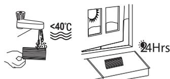
The pre-motor filter should be washed after every five bin empties. Wash under hand warm water. Remove excess water and leave to dry for 24 hours. When completely dry, refit the filter.
