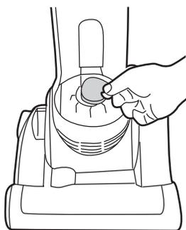
Underneath the dust container you can find the exhaust filter.
