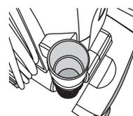
Check for a blockage in the hose socket.
