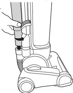
Attach crevice tool to the hose end connector.
