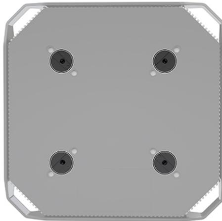
Store the feet on the underside of the computer top cover.
