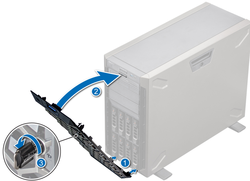
Figure 18. Installing the front bezel
