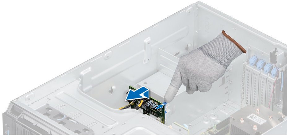
Figure 76. Removing the power interposer board
