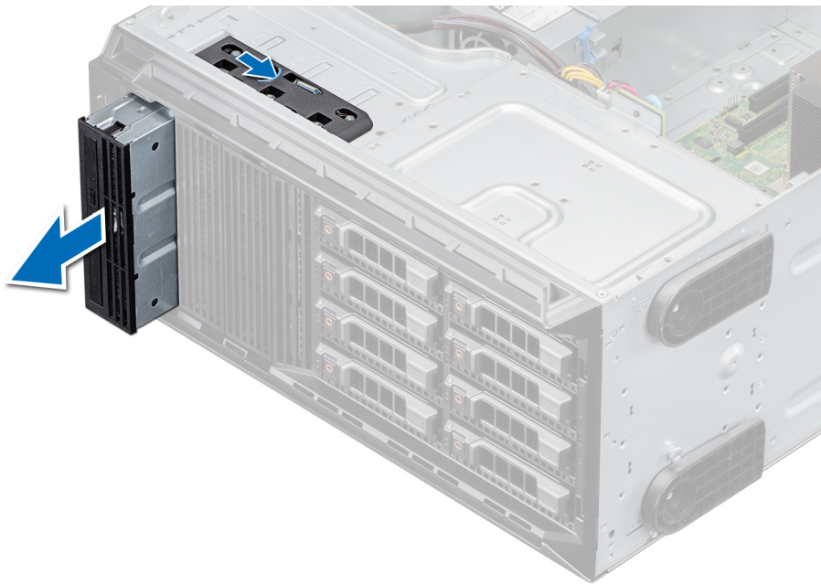
Figure 40. Removing the optical drive
