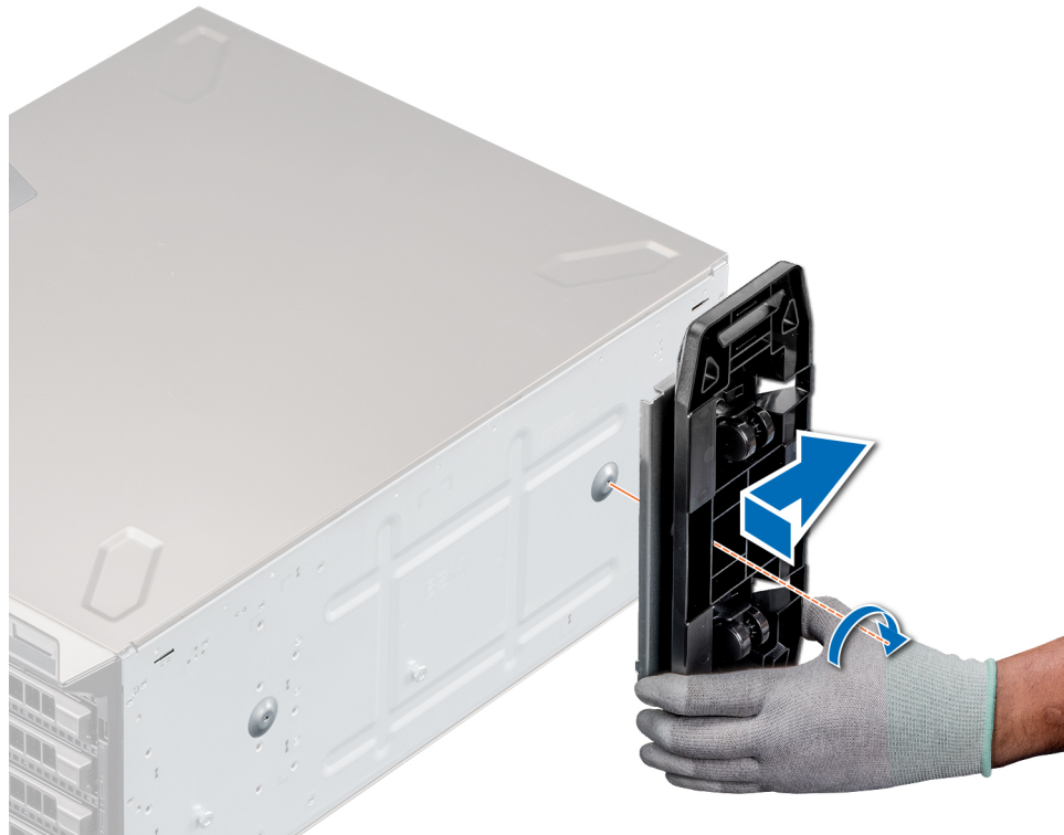
Figure 21. Installing caster wheels
