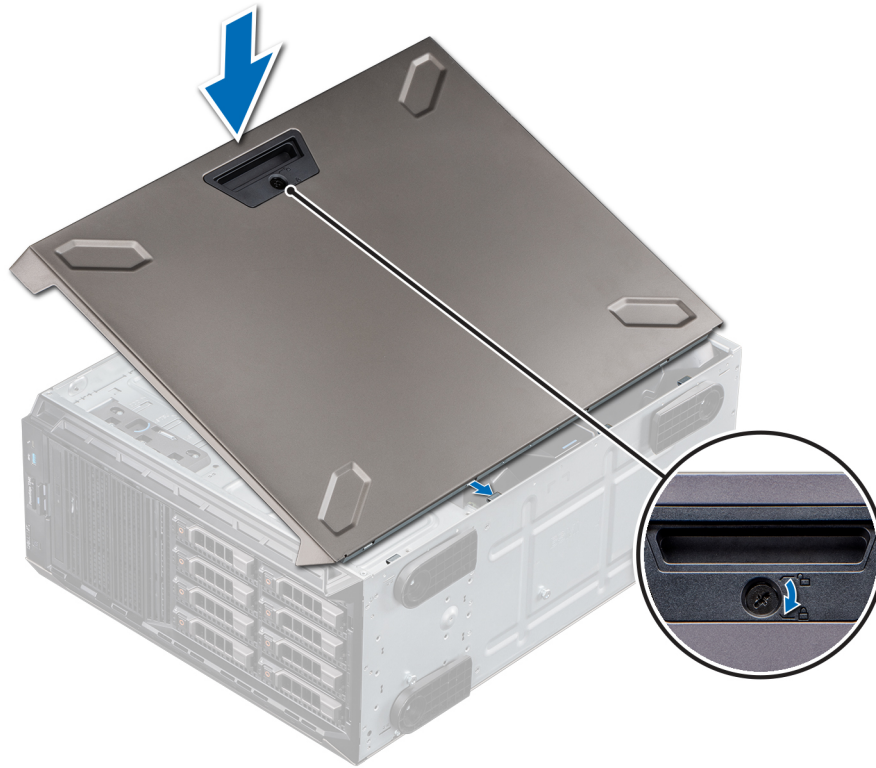
Figure 23. Installing the system cover
