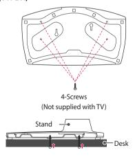
• Screw: M5 x L (\*L: Table depth + 8~10 mm) ex) Table depth: 15 mm, Screw: M5 x L25
