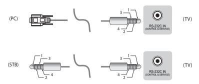
• You need to purchase the phone-jack to RS-232C cable required for the connection between the PC and the TV, which is specified in the manual.
