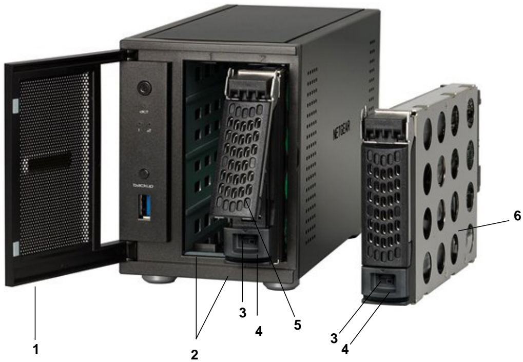
Figure 2. ReadyNAS Ultra 2, Ultra 2 Plus, and Pro 2 drive bay
