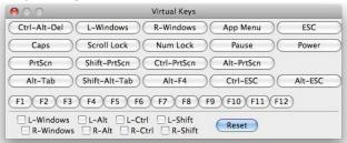
This window allows you to send special key sequences to the attached server, without actually typing them. Many of them are useful combinations, such as Alt-F4, which closes the current window in a Windows operating system.
