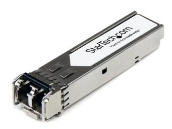
The J9151A-ST is a HP J9151A compatible fiber transceiver module that has been designed, programmed and tested to work with HP brand switches and routers. It delivers dependable 10 GbE connectivity over fiber cable, for 10GBase-LR compliant networks, with a maximum distance of up to 10 km (6.2 mi).
