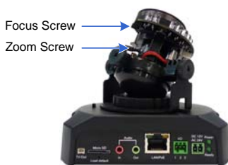
Fixed IP Camera
