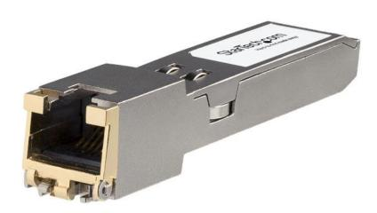
The JL563A-ST is a HP JL563A compatible copper transceiver module that has been designed, programmed and tested to work with HP brand switches and routers. It delivers dependable 10 GbE connectivity over copper cable, for 10/100/1000/10000 compliant networks, with a maximum distance of up to 30 m (98.4 ft).
