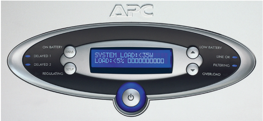
Figure 12. SYSTEM LOAD: <XXXW; LOAD: <XXX% Screen
