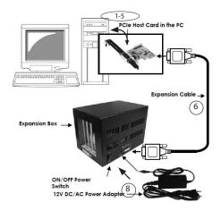
Turn OFF the computer power before installation, and remove the chassis cover from the computer. Similarly, ensure the PEX2PCI4 is not powered at this time.
