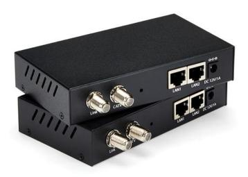
The EOC1110K Gigabit Ethernet over Coaxial Unmanaged LAN Extender Kit (2.4km) includes both end points, and allows you to span a 10/100/1000Mbps Ethernet network over extremely long distances (up to 2.4 km/1.5 mi) while still maintaining high-speed network connectivity.
