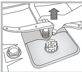
The lower sprayer arm can be removed by pulling it upwards.
