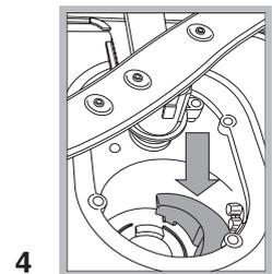
After cleaning the filters, replace the filter assembly and fix it in position correctly; this is essential for maintaining the efficient operation of the dishwasher.
