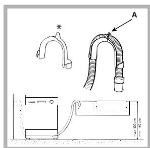
The special plastic elbow\* makes it easier to find the best layout: fix the elbow to the wall securely in order to prevent the outlet hose from moving and spilling the dirty water. The part of the hose marked with the letter A should be between 40 and 100 cm above the ground
