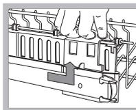
If the rack is fitted with “Dual Space” handles\* (*see figure*), pull out the upper rack until it reaches its stop point, grip the handles at the sides of the rack and move it upwards or downwards, then slowly let it fall back
