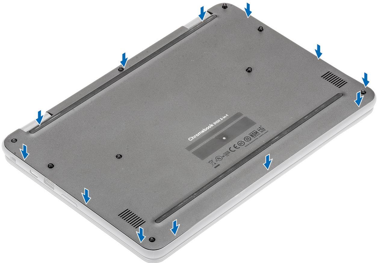
2 Tighten the nine captive screws to secure the base cover to the computer.
