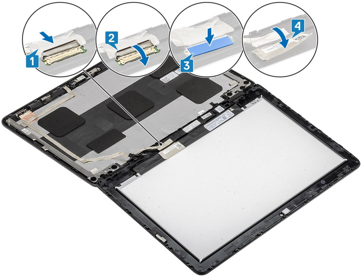
3 Carefully flip the display over on to the display panel.
