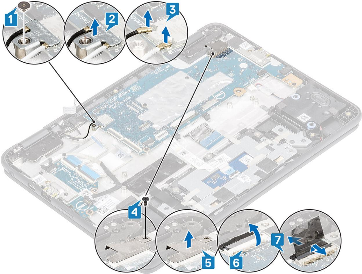
7 Lift the system board bracket away from the computer.
