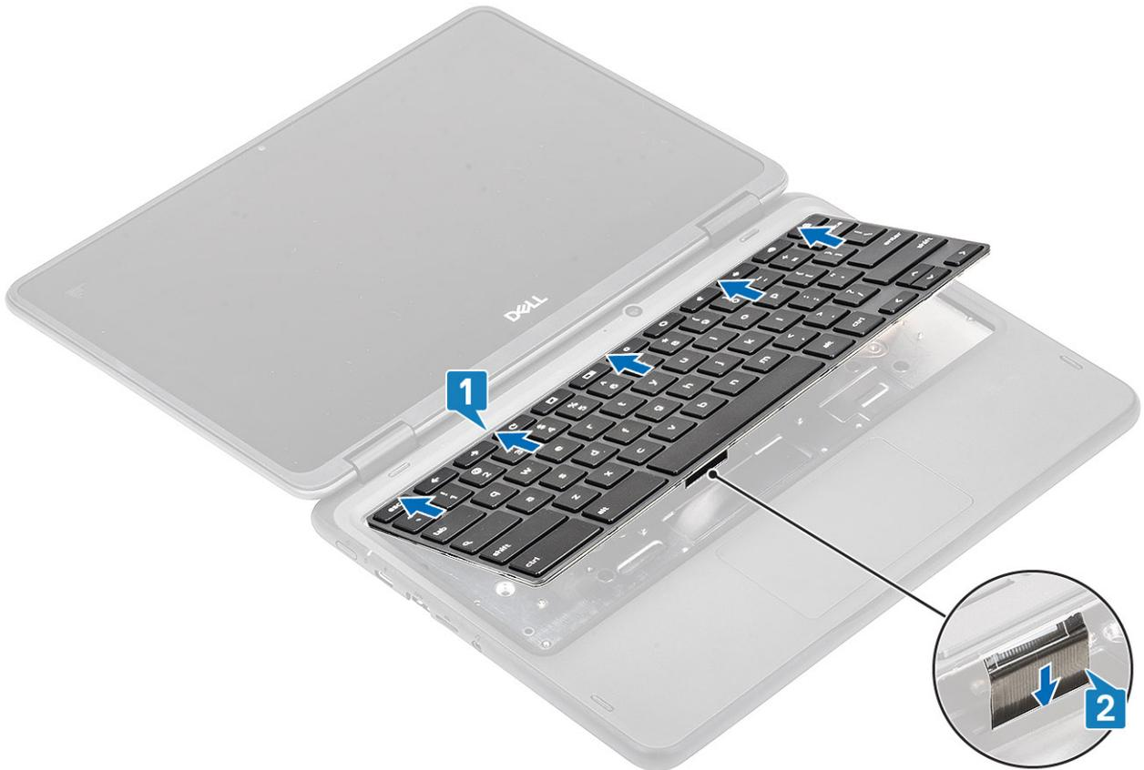
2 Press the keyboard until it clicks into place and then close the LCD fully before turning the system over [1, 2]
