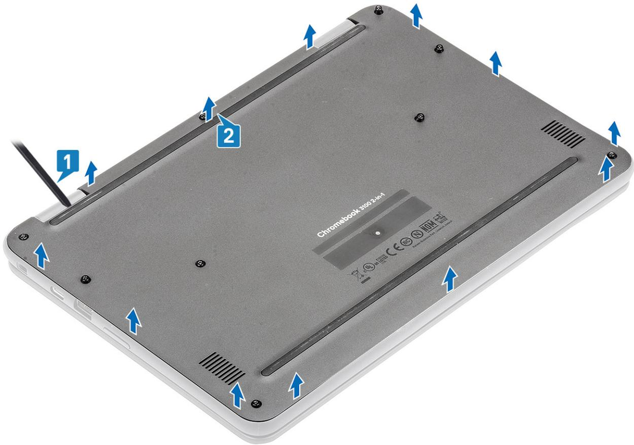
① **NOTE:** While removing the base cover, on-site technicians must take care to remove the base cover carefully. There are prying recess points next to the left and right hinges which ease the disassembly procedure. With the help of a plastic scribe, pry open from the top left side of the base cover, continue working your way around the left and right side of the base cover, then remove the base cover from the system.
