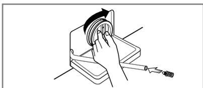
4. After cleaning, turn the pump filter and insert
