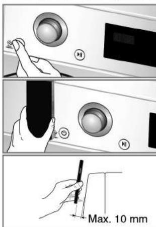
1. Press the Power button to turn on the washer. Do not press any other buttons or turn the cycle selector knob.
