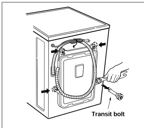
1. Unscrew the 4 bolts with the spanner supplied.
