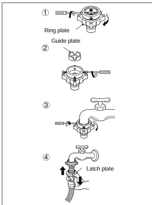
1. Unscrew the adapter ring plate and the 4 adapter retaining screws.
