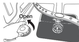
2. If you are filling the container for the first time, fill 2/3 of its volume with water (around 1 liter).
