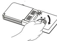
The rinse aid is released during the final rinse to prevent water from forming droplets on your dishes that can leave spots and streaks. It also improves drying by allowing water to run off the dishes.
