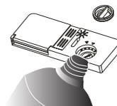
3. Replace the cap by inserting it aligned with "Open" arrow and turning it to the closed (right) arrow.
