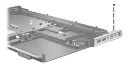
Where used: One screw that secures the power connector and bracket to the base enclosure
