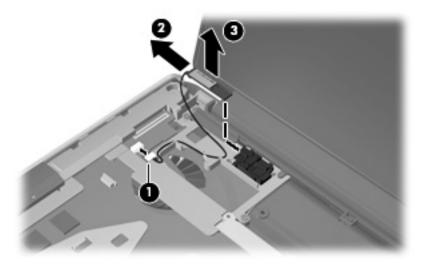
Reverse this procedure to install the Bluetooth module.
