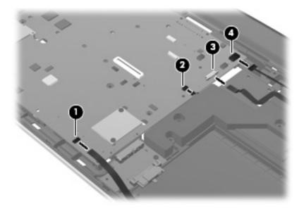
2. If necessary, disconnect the hard drive connector cables from the system board.
