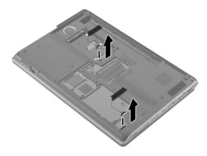
3. Remove the three Phillips PM2.5×5.0 screws that secure the system board to the base enclosure.
