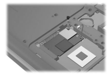
Where used: One screw that secures the TV tuner module to the system board
