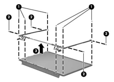
The left and right sides of the display hinge assembly are secured to a bracket **1** using four PM2.5×4.0 screws **2** as shown in the following image.
