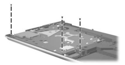
**Where used:** 3 screws that secure the system board to the base enclosure
