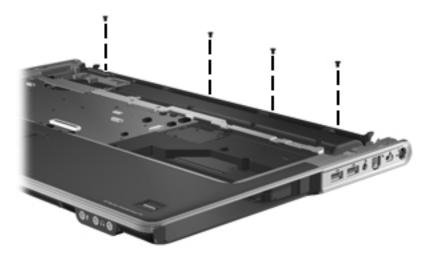
Where used: 4 screws that secure the top cover to the base enclosure (along top of base enclosure)
