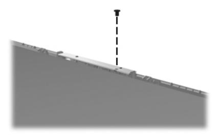
**Where used:** One screw that secures the webcam/microphone module to the display bezel on computer models equipped with flush glass display assemblies
