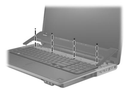
Where used: 4 screws that secure the keyboard to the top of the computer
