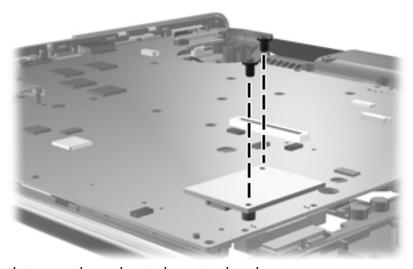
Where used: 2 screws that secure the modem to the system board
