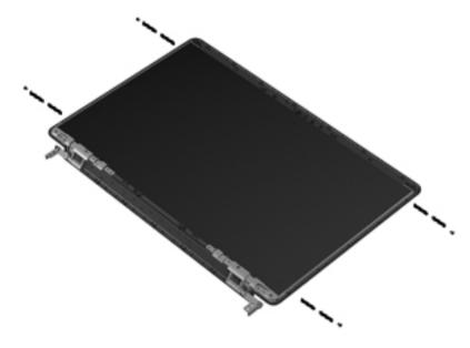
**Where used:** 4 screws that secure the display hinges to the display panel on computer models equipped with flush glass display assemblies
