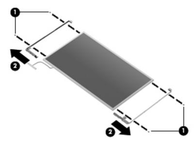
30. If it is necessary to remove the display panel cable, remove the adhesive plastic strip ● from the display panel cable, and remove the display panel cable ②. Remove the tape ③ that secures the cable to the display panel. The display panel cable is available using spare part number 516307-001.
