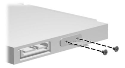
Where used: 2 screws that secure the optical drive bracket to the optical drive
