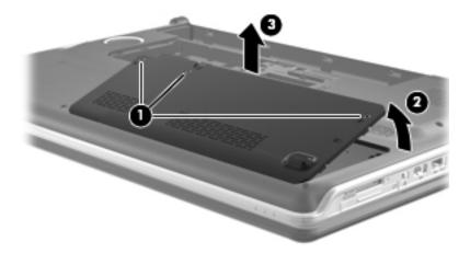
Reverse this procedure to install the secondary hard drive cover.
