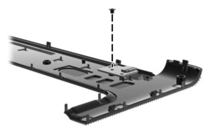
Where used: One screw that secures the power button board to the switch cover
