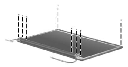
**Where used:** 8 screws that secure the display panel to the display enclosure on computer models equipped with BrightView display assemblies
