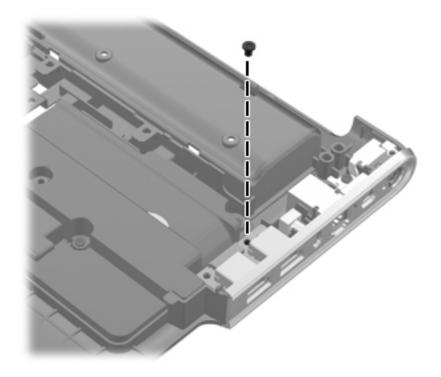
Where used: One screw that secures the USB board to the base enclosure
