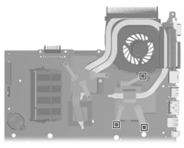
Where used: 3 screws that secure the fan/heat sink to the system board
