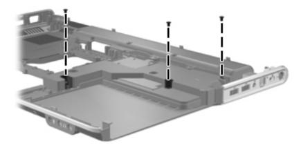
Where used: 3 screws that secure the subwoofer to the computer
