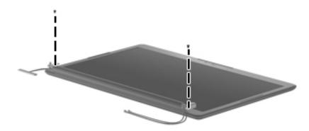
**Where used:** 2 screws that secure the display bezel to the display enclosure on computer models equipped with BrightView display assemblies
