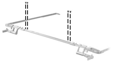
**Where used:** 4 screws that secure the display hinges to the hinge bracket on computer models equipped with flush glass display assemblies
