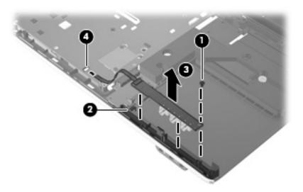
Reverse this procedure to install the audio/infrared board.
