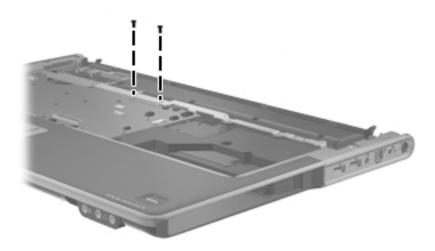
Where used: 2 screws that secure the top cover to the top of the computer
