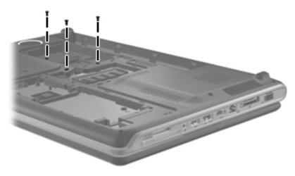
**Where used:** 3 screws that secure the keyboard to the base enclosure
