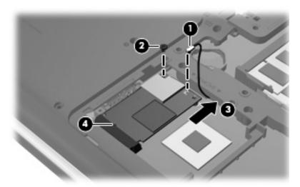
Reverse this procedure to install the TV tuner module.
