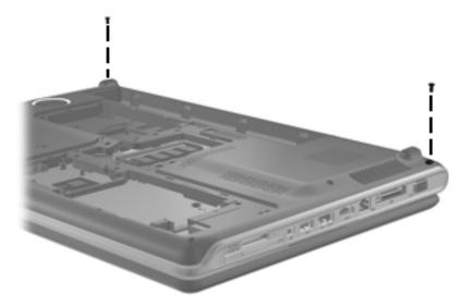
Where used: 2 screws that secure the switch cover to the computer
