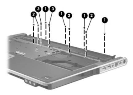
5. Remove the top cover by lifting it straight up. Reverse this procedure to install the top cover.
