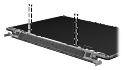
**Where used:** 4 screws that secure the display hinges to the display hinge bracket on computer models equipped with flush glass display assemblies
