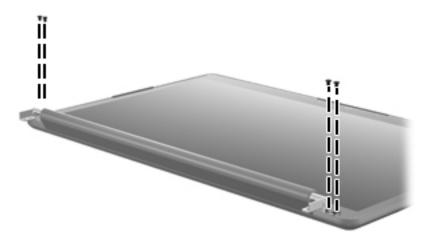
**Where used:** 4 screws that secure the display bezel to the display enclosure on computer models equipped with flush glass display assemblies
