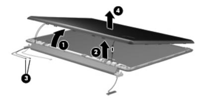
11. If it is necessary to remove the hinge cover, remove the four Phillips PM2.5×5.0 screws • that secure the hinge cover to the display assembly, and then remove the cover • The hinge cover is available using spare part number 537844-001.
