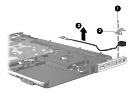
Reverse this procedure to install the power connector cable.
