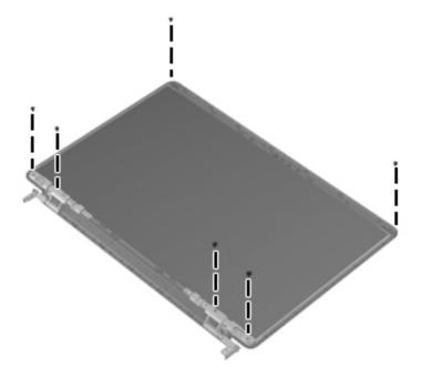
**Where used:** 6 screws that secure the display hinges to the display panel on computer models equipped with flush glass display assemblies
