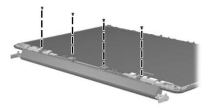
**Where used:** 4 screws that secure the hinge cover to the display enclosure on computer models equipped with flush glass display assemblies
