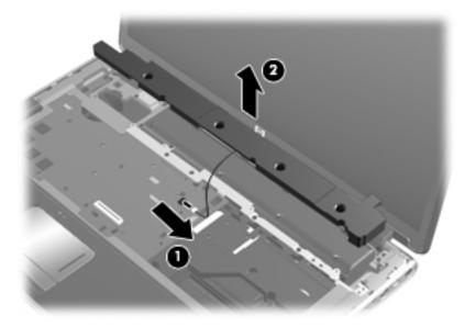
Reverse this procedure to install the speaker assembly.
