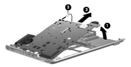
6. If it is necessary to remove the optical drive board from the system board, pull the optical drive board straight off the system board. The optical drive board is available using spare part number 519481-001.
