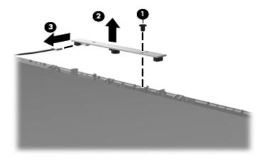
15. Disconnect the display panel cable from the display panel. The display panel cable is available using spare part number 516307-001.
