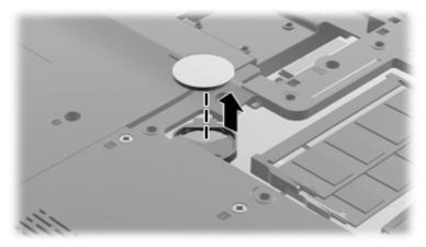
Reverse this procedure to install the RTC battery. Be sure the RTC battery is installed with the "+" sign facing up.
