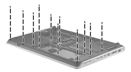
Where used: 11 screws that secure the top cover to the base enclosure
