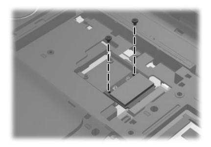
Where used: 2 screws that secure the WLAN module to the system board
