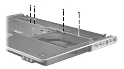
Where used: 4 screws that secure the top cover to the top of the computer
