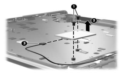
Reverse this procedure to install the modem module.
