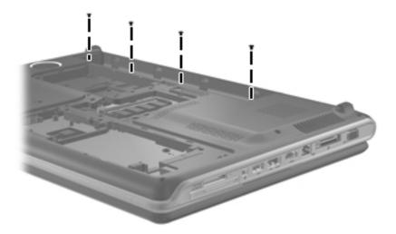
Where used: 4 screws, located inside the battery bay, that secure the switch cover to the computer
