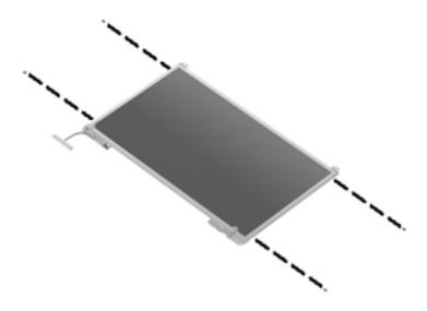
**Where used:** 4 screws that secure the display panel to the display enclosure on computer models equipped with BrightView display assemblies
