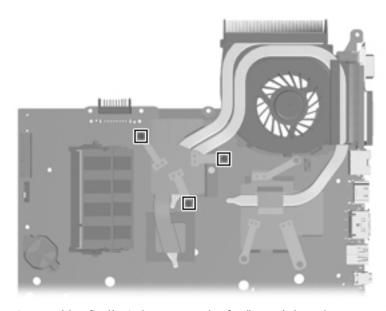
Where used: 3 screws (secured by C-clips) that secure the fan/heat sink to the system board
