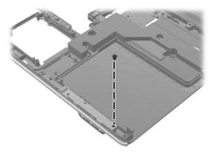
Where used: One screw that secures the audio/infrared board to the base enclosure
