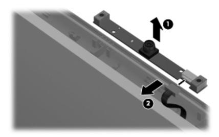
24. If it is necessary to replace the display panel, remove the two Phillips PM2.5×6.0 screws **1** from the top corners and the six Phillips PM2.5×6.0 screws **2** from the display hinges. The display panel is available using spare part number 516303-001.
