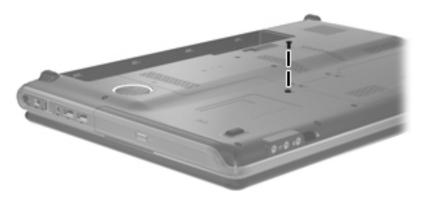
Where used: One screw that secures the optical drive to the computer
