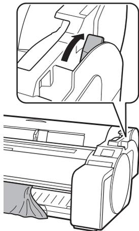
Push the release lever to the back side.
