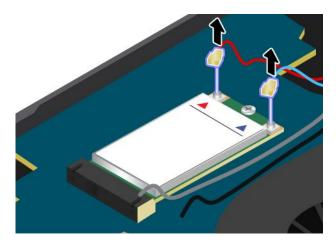
5. Remove the screw 1. The wireless WAN card pops up. Remove the WAN card 2.
