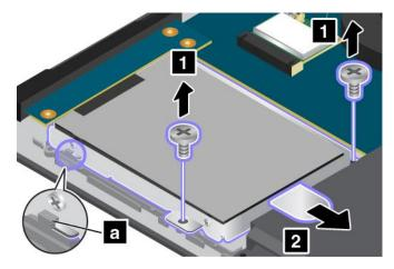
5. Remove the hard disk drive or solid-state drive by lifting the tab.
