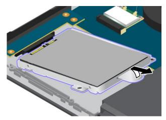
6. Place the new hard disk drive or solid-state drive into the drive bay.
