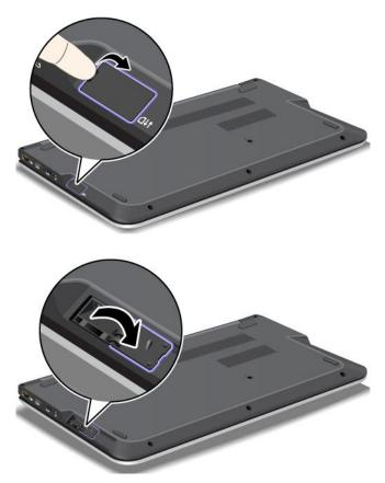
To install the SIM card, go to step 5. If you are replacing a SIM card, please continue.
