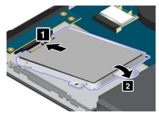
7. Slide the hard disk drive or solid-state drive horizontally and firmly into the connector **1**. Ensure that the hard disk drive or solid-state drive is correctly seated in the bay and secured by the hook **a**. Then reinstall the screws **2**.
