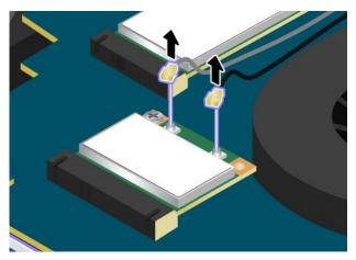
5. Remove the screw 1. The card pops up. Remove the card 2.
