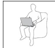
When your computer is turned on or the battery is charging, the base, the palm rest, and some other parts may become hot. The temperature they reach depends on the amount of system activity and the level of charge in the battery.
