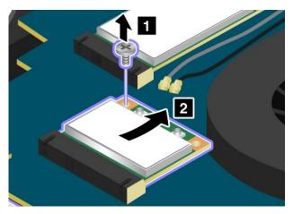
6. Align the contact edge of the new card with the corresponding socket **1**. Pivot the card until you can snap it into place. Secure the card with the screw **2**.
