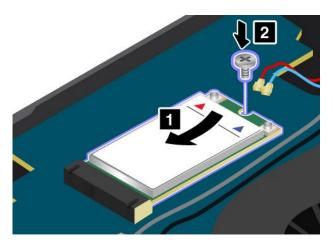
7. Connect the antenna cables to the new WAN card.
