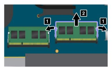
Place the notched end of the new memory module toward the contact edge side of the memory slot and insert the memory module into the slot 1 at an angle of about 20 degrees. Pivot the memory module downward until it snaps into place 2. Ensure that the memory module is firmly installed in the slot and cannot be moved easily.
