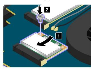
7. Connect the antenna cables to the new card.
