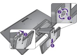
• Release the thumbscrew on the bottom of the monitor base. Then pull the stand backward away from the stand and detach the monitor base as illustrated.
