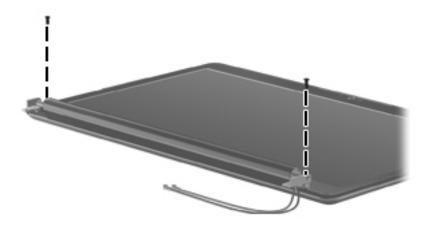
Where used: 2 screws that secure the display bezel to the display
