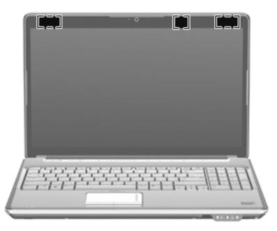
For optimal transmission, keep the areas immediately around the antennas free from obstructions.
