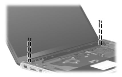
Where used: 4 screws that secure the display assembly to the computer
