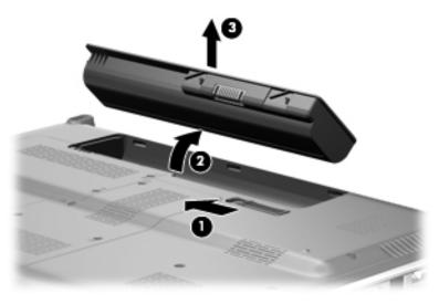
To insert the battery, insert the rear edge of the battery into the battery bay and pivot the front edge of the battery downward until it is seated. The battery release latch automatically locks the battery into place.
