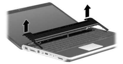
5. Move the switch cover back so that it rests on the display.
