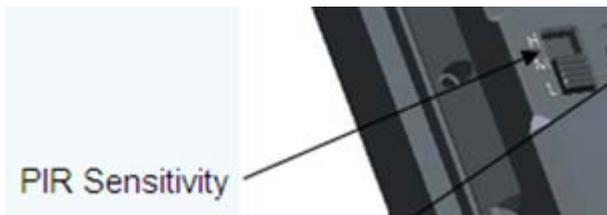
This camera has 3 sensitivity levels. Choose “H” (“H” means high sensitivity) when the weather is hot. Choose “M” (“M” means middle sensitivity) when the weather is normal, and choose “L” (“L” means low sensitivity) when the weather is cold. If you want the camera to detect long distance coverage, or to sense very small animals, please always put the Switch at “H”.
