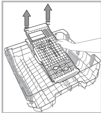
The upper rack can be adjusted for height based on requirements: high position to place bulky crockery in the lower rack and low position to make the most of the tip-up dispensers/sectors by creating more space upwards.
