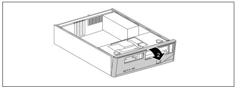
► Fold the front panel in the direction of the arrow (2) and remove it from the casing.
