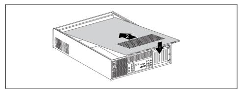
Place the cover on the casing (1) and push it into place in the direction indicated by the arrow (2).
