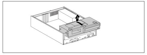
▶ Use the plastic handle to lift the drive cage out of the casing (3).
