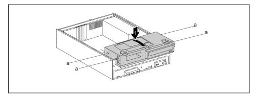
Insert the drive cage on the plastic handle into the casing (1). When doing so, ensure that the guides (a) are at the height of the corresponding openings on the casing.
