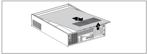
▶ Pull the cover a small distance in the direction indicated by the arrow (2) and remove it (3).
