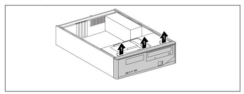
Lift the locking lugs on the front panel (1).
