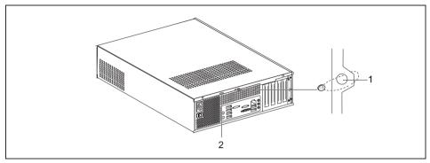
1 = Holes for padlock/lead-seal
