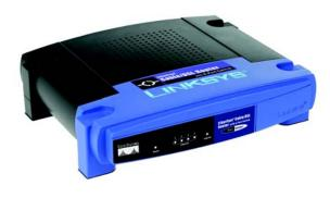
Think of the EtherFast Cable/DSL Router with 4-Port Switch as a kind of "splitter" for your Internet connection. Just connect your DSL or Cable Modem to the Router, and all the computers in your household can share the Internet—all at the same time. The built-in 4-port switch lets you attach four local PCs directly, or daisy-chain out to more hubs and switches as your network grows.
