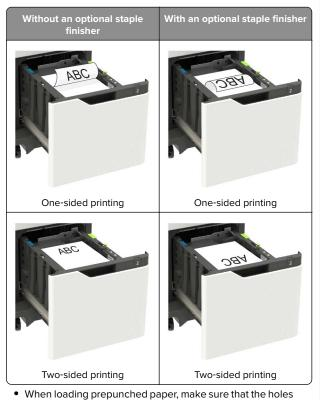
• When loading prepunched paper, make sure that the holes on the long edge of the paper are against the right side of the tray.
