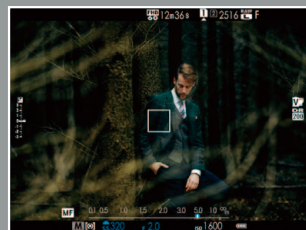
The Depth of Field Scale, displayed as a blue bar in the distance index, gives a visual guide when manually pre-focusing.
