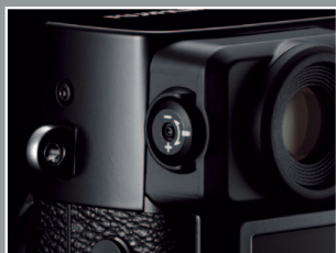
Optical viewfinder diopter correction is not only available on the EVF, but also when using the OVF and ERF.
