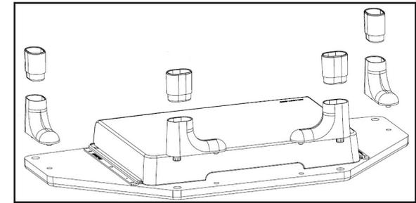
*Inserting the Extenders into the Legs*
