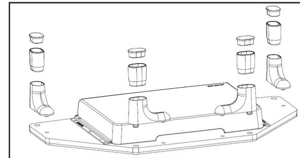
*Inserting the Rubber Feet into the Legs*
