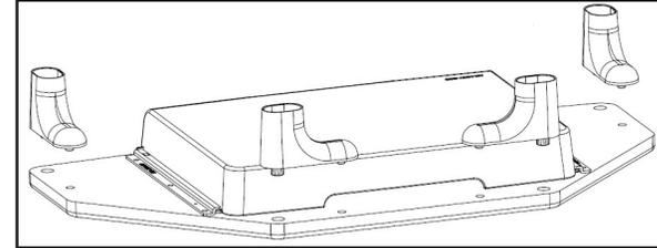
*Inserting the Legs into the Platform*
