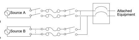
Source B relays are engaged. Source B provides power to the attached equipment.
