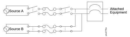
**NOTE:** The entire switching process (described in step 2) takes a maximum of 10 milliseconds (ms) at high sensitivity, and 12 ms at low sensitivity. (This applies to both 50 Hz and 60 Hz sources.)
