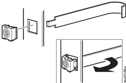
From inside the enclosure, insert the cage nut into the square hole.
