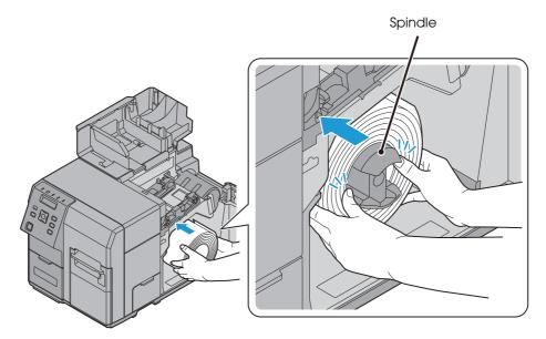
Pull out the end of roll paper about 300 mm {11.8"} in order for the paper auto feeding in the step 12 to go smoothly.
