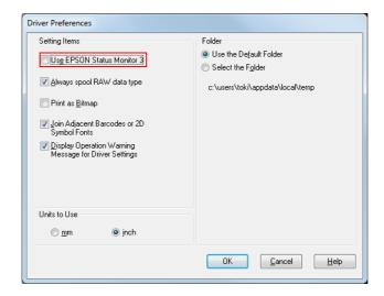
(EPSON Status Monitor 3) and (Monitoring Preferences) are displayed in (EPSON Status Monitor 3 Settings) on the Driver Utilities window.
