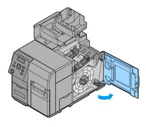
Pull out the roll paper flange while holding the release lever of the roll paper flange between your fingers.
