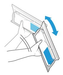
4 Push all the ink cartridges of the four colors gently into the product until they click in place. Check the color of the ink cartridge label and of the ink cartridge holder label, and set the cartridges to each matching color.
