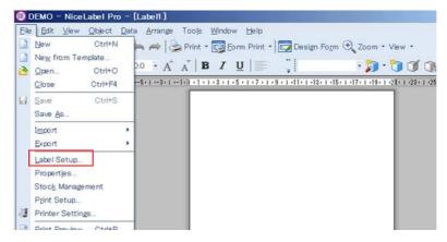
The "Label Setup Wizard" window or the "Label Setup" window appears. Select "Epson TM-C7500 for NiceLabel" and click (Properties...).
