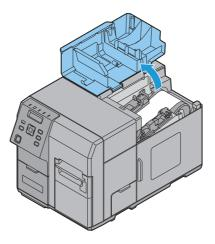
**?** Pull the front cover open lever at the paper feed slot.
