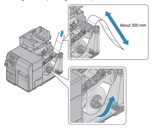
**7** Attach the roll paper flange to the spindle while holding the release lever of the roll paper flange between your fingers. Push the flange to the bottom to align it with the roll paper width.
