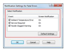
• Ambient Temperature Error: When the printer temperature is high
