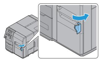
2 Insert the rewinder's power transmission gear into the cover opening.
