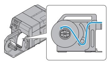
Fix the tip of the paper to the core or insert it into the gap of the rotation axis.
