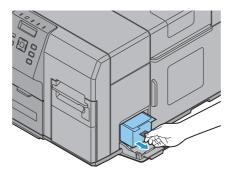
4 Put the maintenance box into the plastic bag for disposal of used maintenance box.
