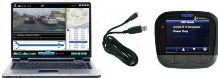
Use the USB port on the side of the device to connect the device to your computer. When connected you will be given two options: **Connect to Computer** or **Power Only**.
