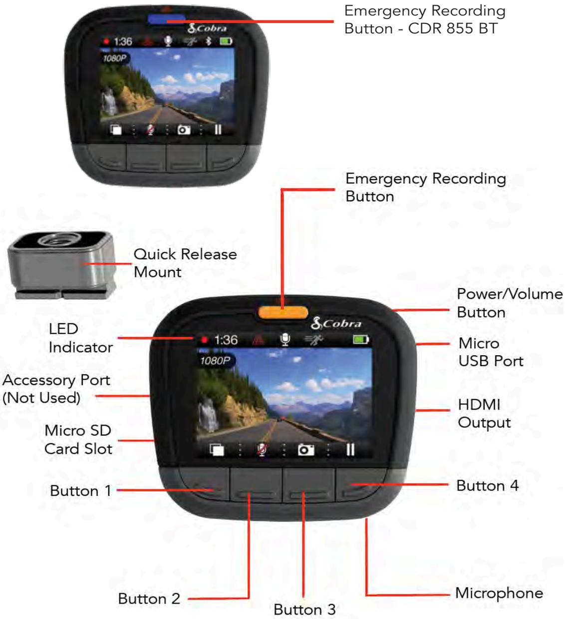
The functions of Buttons 1-4 are indicated by the icon directly above each button and change depending on the state of the unit.
