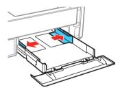
3 Insert paper with the printable side down and slide the edge guides against the paper, but not too tightly.
