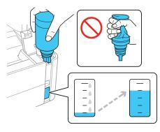
**Note:** If ink does not flow from the bottle, lift and reinsert the bottle.
