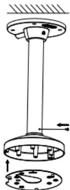
Figure 2-17 Install the Adapter Plate
