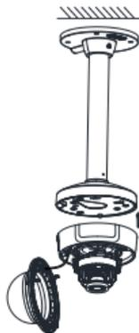
Figure 2-18 Secure the Camera
