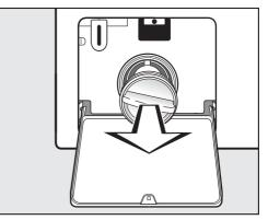
Remove the drain filter completely.
