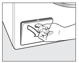
Open the drain pump access panel.
