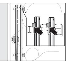
Secure the transit bars to the back of the washing machine. Make sure the top catch is located above the holder.
