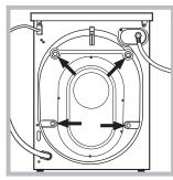
Remove the 4 protective screws and the rubber bush with the respective spacer, situated on the rear of the appliance (see also the installation leaflet).
