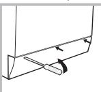
1. using a screwdriver, remove the cover panel on the lower front part of the washing machine (see figure);
