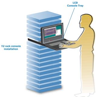
The LCD Console Tray can be connected directly to your PC/server or to a group of PCs/servers via an Avocent KVM switch.
