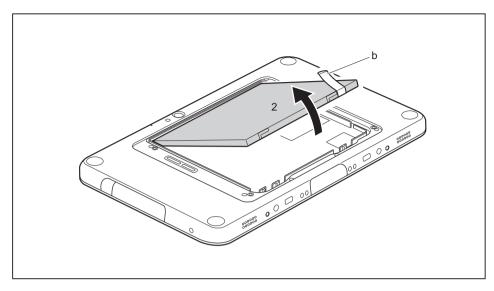
▶ Pull on the pulling aid (b) and lift the battery out of the battery compartment in the direction of the arrow (2).
