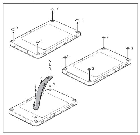
▶ Remove the covers from the screw holes on the rear of the tablet PC (1).
