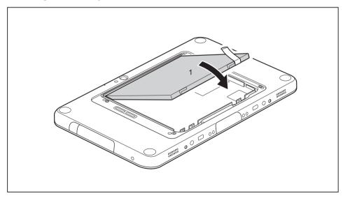
▶ Position the battery at the edge of the battery compartment and insert the battery in the battery compartment (1).
