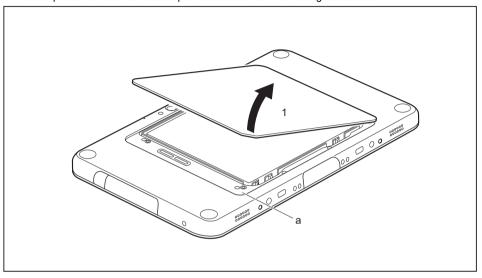
► Reach into the opening (a) with one finger and take off the battery cover in the direction of the arrow (1).
