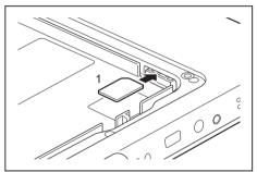
Insert the SIM card into the slot (1) as shown and with the chip downwards.
