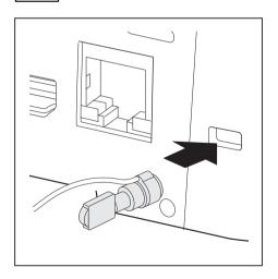
If the Tablet PC is connected to the cradle (optional): Fit the Kensington Lock cable to the fixture on your cradle.
