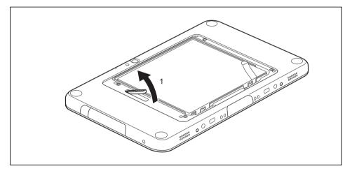
Remove the cover (1) in the battery compartment.
