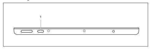
▶ Press the ON/OFF button (1) for about one second to switch the device on.
